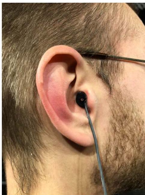
Fig. 3. Microphone inserted in the subject's ear.
