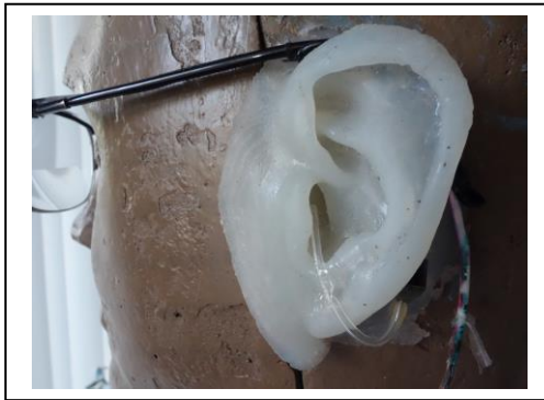
Figure 6: A probe microphone glued just inside the ear canal of the author’s model head. The model has castings of his ears all the way to the eardrum, and the eardrum impedance modelled with a resistance tube. The free-field frontal response at the eardrum closely matches his own head.
