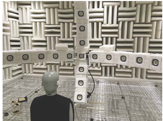
Fig. 2. A picture of the RIEC anechoic room at Tohoku University, the reference room used in this study. The Head and Torso Simulator (the Brüel & Kjær 4100D) is located at the center of the loudspeaker array for the binaural recording of the 22.2 and two-channel reproduced orchestral music pieces.
