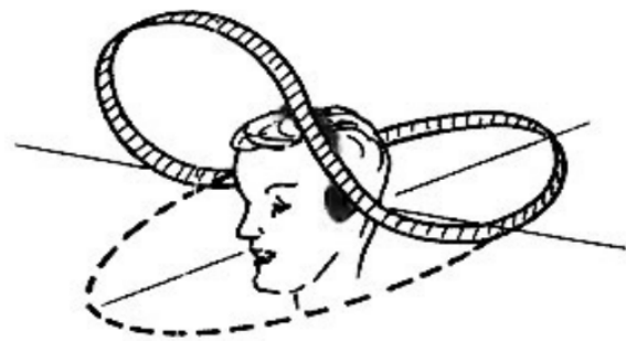
Fig. 1: Illustration of commonly perceived trajectory in headphone listening to a binaural recording of a sound moving around the listener’s head in the horizontal plane (from [15]).
