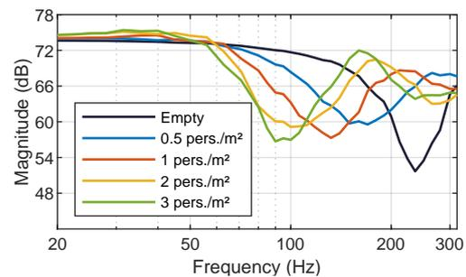
**Fig. 9:** Frequency response at 20 m, for a source at 4.6 m height, for different audience densities.
