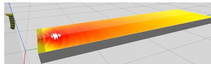
**Fig. 3:** Soundvision 3D plot of an array made of 8 L-Acoustics Kara II
