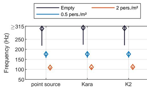
**Fig. 13:** Variability of the first notch frequency as a function of the source type (point source at 4.6 m height or line sources of Kara and K2), for several audience densities.
