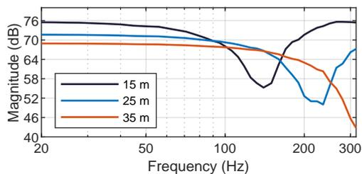
**Fig. 7:** Frequency response at three distances from the source (point source at 6.3 m height), without audience.
