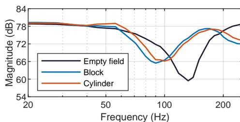
**Fig. 4:** Comparison of the frequency response at 10 m with two models for the human body in a small field of 15 m long per 8 m wide, with a density of 2 pers./m<sup>2</sup>.
