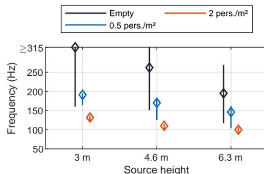
**Fig. 10:** Variability of the first notch frequency as a function of the source position, for several audience densities.
