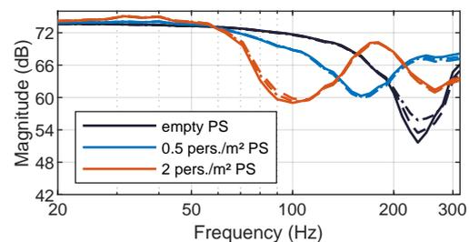
**Fig. 12:** Frequency response of a point source (PS) at 4.6 m, continuous line, and of line sources, dashed line for Kara, dash-dotted line for K2, at 20 m, for several audience densities.
