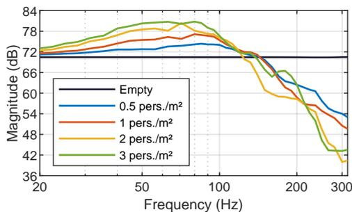
**Fig. 14:** Frequency response at 20 m for a source on the ground, with several audience densities.
