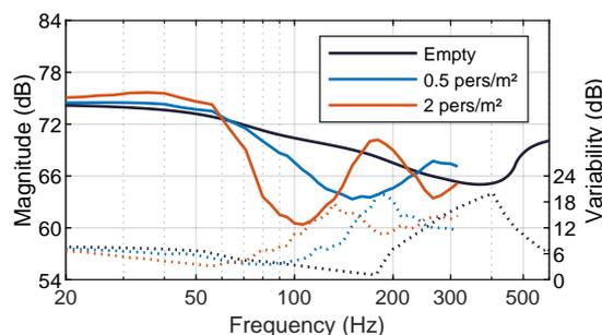
**Fig. 11:** Mean frequency response on the whole listening area for several audience densities, source at 4.6 m (left axis - continuous lines), corresponding variability (right axis - dotted lines).
