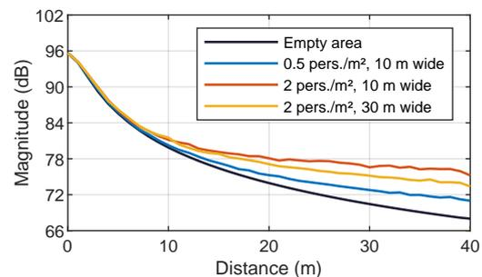
**Fig. 16:** Sound pressure level decrease with distance for a ground source, with several audience densities and listening area widths.
