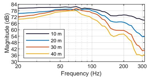
**Fig. 15:** Frequency response at several distances, for a source on the ground with a density of 2 pers./m<sup>2</sup>.
