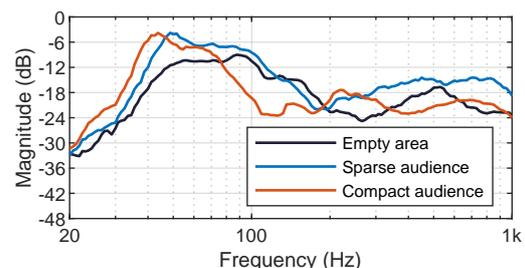
**Fig. 1:** Measurement of the house-right line source, at 53 m distance, microphone at 1.7 m height, without an audience and with two audience densities.
