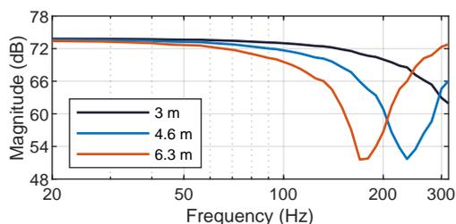
**Fig. 8:** Frequency response at 20 m from the source flown at three different heights, without audience.
