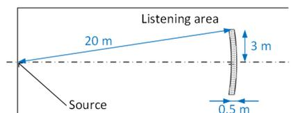
**Fig. 6:** Top view of the listening area showing the annular segment used to calculate the mean frequency response at 20 m.
