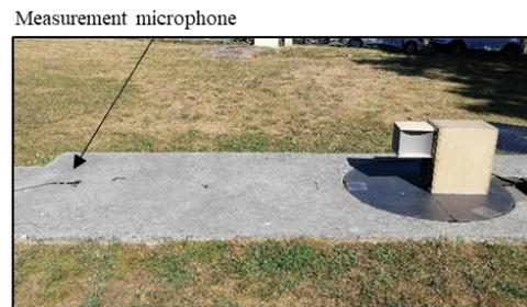
Fig. 5: Outdoor measurement setup for acoustic loss measurement.
