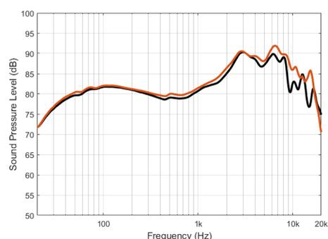
**Fig. 4:** Average of the left and right channels of a Beyerdynamic DT-990 Pro headphone after eq was applied to meet the “2013 Harman Target”
