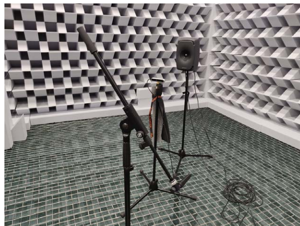
Fig. 3. Measurement setup in the large anechoic chamber of the Aalto Acoustics Lab.
