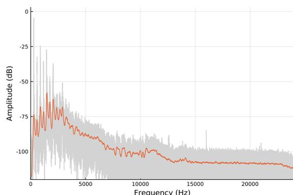
**Fig. 8:** Noise level calculation using moving median on the spectrum. Light colored lines are the power spectrum of the sound A1, and darker curve is moving median of the spectrum.
