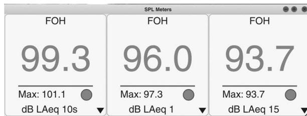
Fig. 1. Example of triple equivalent continuous sound pressure level ( $L_{eq}$ ) time frame monitoring during a recent live event.
