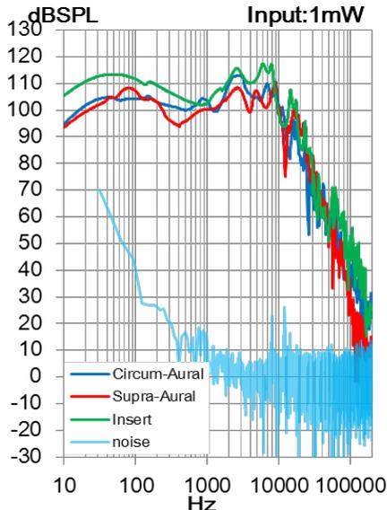
Figure 11. HATS output vs. background noise spectrum: Instant Value: Industry Standard HATS
