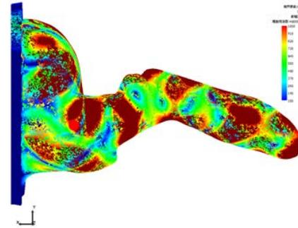
Figure 15. SPL Simulation inside of human ear canal: (46 kHz)
