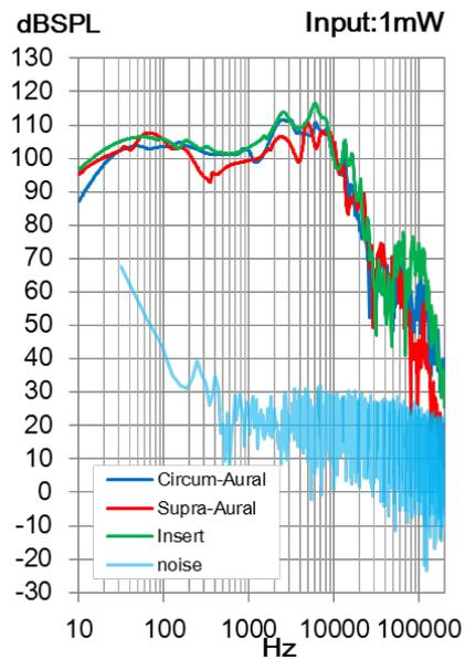
Figure 9. HATS output vs. background noise spectrum Instant Value:
