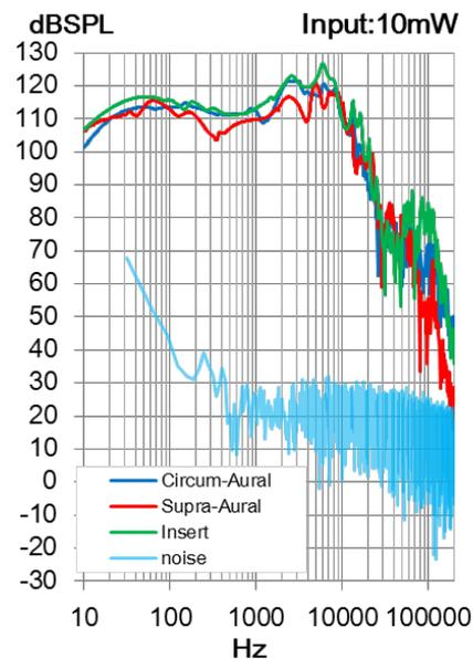
Figure 12. HATS output vs. background noise spectrum: Instant Value: HATS Prototype 2
