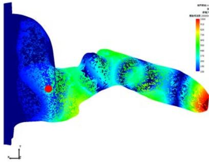
Figure 13. SPL Simulation inside of human ear canal: (20 kHz)
