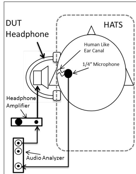
Figure 5. Measurement system block diagram
