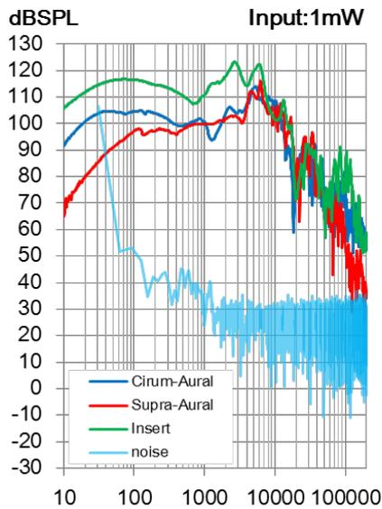
Figure 10. HATS output vs. background noise spectrum: Instant Value : HATS Prototype 1
