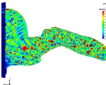
Figure 17. SPL Simulation inside of human ear canal: (200 kHz)
