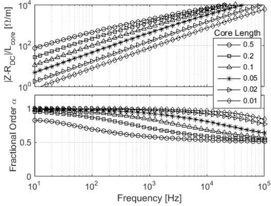
**Fig. 5:** FEM simulated magnitude of AC impedance (top) and fractional order  $\alpha$  for finite coils of different lengths. Shorter coils have higher transition frequencies ( $\alpha = 0.75$ ) than longer coils. The transition bandwidth is roughly 3 decades for all lengths.
