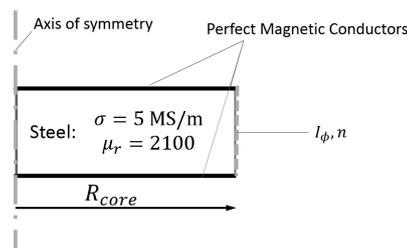
**Fig. 2:** Simulation setup for the infinite core simulations. The infinite coil is approximated by a short coil with perfect magnetic conductors at the truncations. Mathematically, the perfect magnetic conductors allow magnetic flux lines to start and terminate, which is not possible physically.
