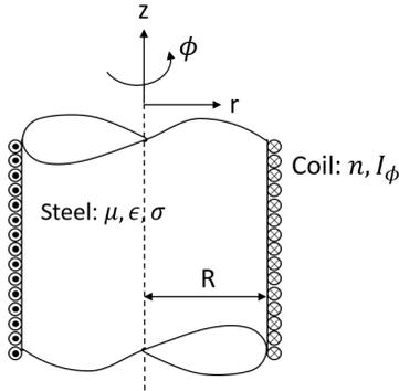
**Fig. 1:** A diagram of the infinite coil around an infinite core. The core has radius  $R$  and its material properties are given by  $\mu$ ,  $\epsilon$ , and  $\sigma$ . The coil is infinitely thin and carries a current in the  $\phi$ -direction with a turn density of  $n$  turns per unit length of the core. The core's axis lines up with the  $z$ -axis, and the sign of  $\phi$  is given by the right-hand rule.
