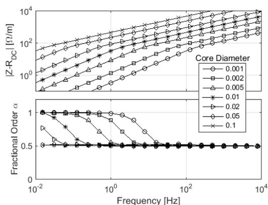
**Fig. 4:** FEM simulations (solid lines) and analytical solution (markers) for the AC impedance magnitude (top) and the fractional order  $\alpha$  (bottom) of infinite coils of different diameters.
