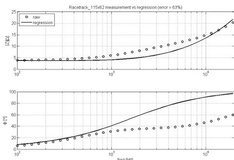
**Fig. 8:** Driver D - Raw impedance amplitude (top) and phase (bottom) vs. complex regression (i.e. fractional order model).
