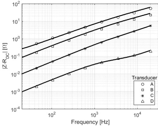
**Fig. 6:** FEM simulations (solid lines) and measurements (markers) of the AC impedance of Drivers A to D. **Note:** Impedance values of transducer D are plotted lower by a factor of 100 for better legibility.
