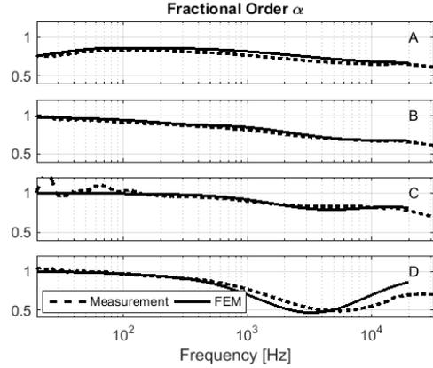
**Fig. 7:** FEM simulations (solid) and measurements (dotted) of fractional order  $\alpha$  of the magnitude of the AC impedance of transducers A to D.
