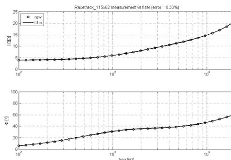
**Fig. 10:** Driver D - Log-Log plot of raw impedance data vs. optimized filter with 8 R-L cells.
