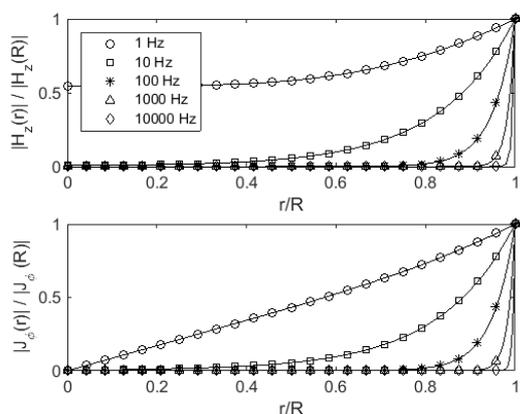
**Fig. 3:** Comparison of FEM simulation (solid lines) and analytic solution (markers) for the normalized absolute induced magnetic field strength (top) and the normalized absolute induced current density (bottom).
