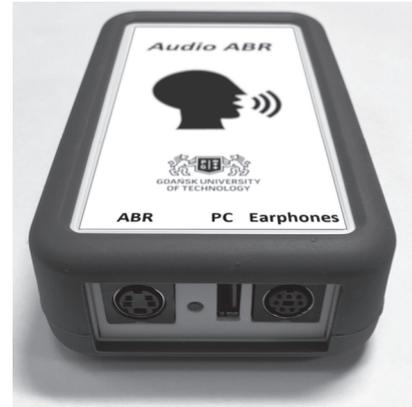
Figure 4. Audio ABR device, the speech-oriented version
