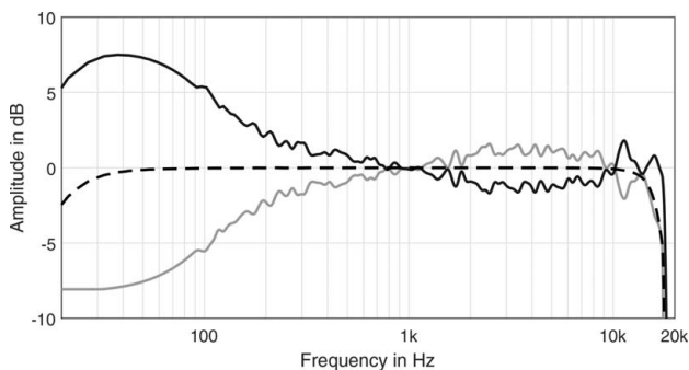
Fig. 4. Transfer function (gray) and inverse filter (black) for a Neumann KM120 microphone; the dashed line shows the compensation result of the inverse filter on the transfer function.
