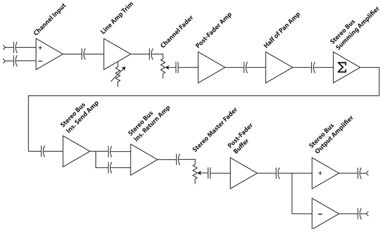
Fig. 3. Test circuit block diagram. One channel shown.
