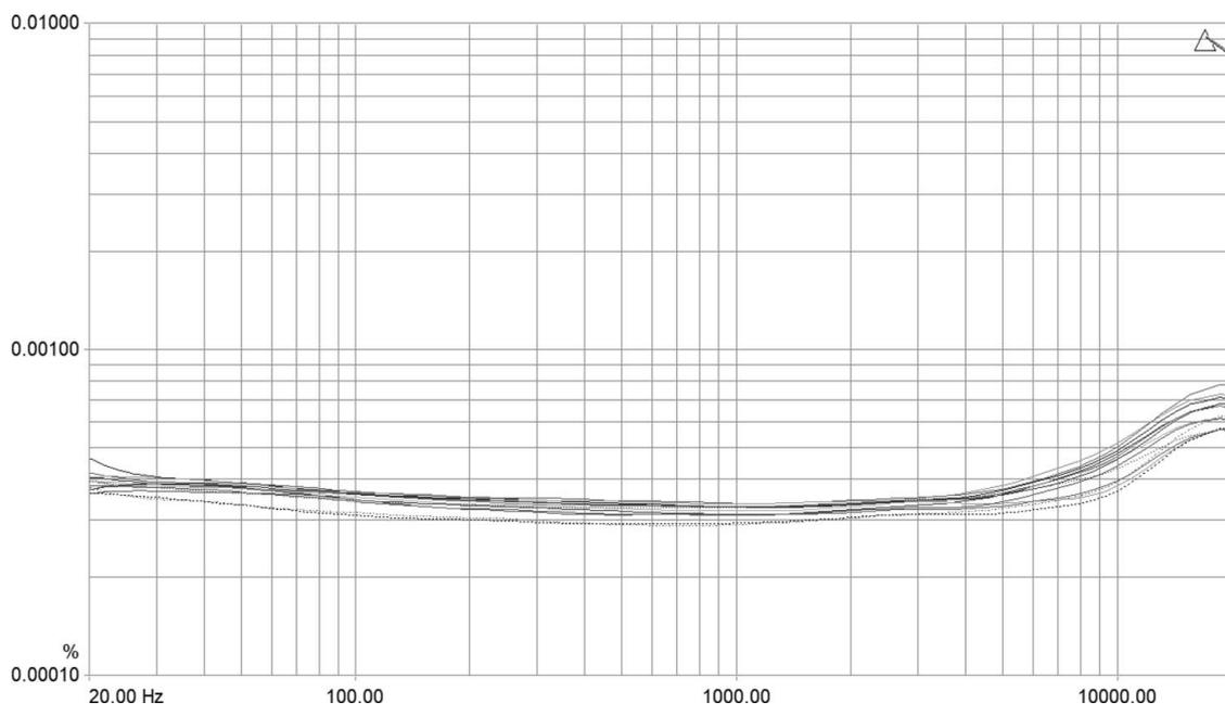
Fig. 5. Total harmonic distortion (THD) sweeps at +10 dBu.
