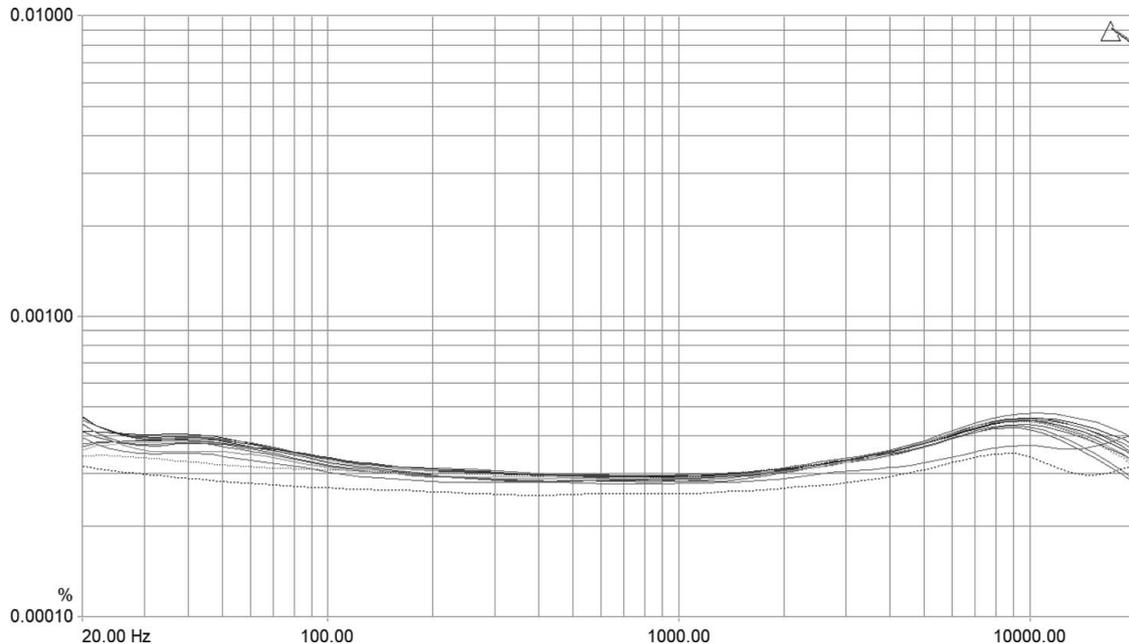
Fig. 4. Total harmonic distortion (THD) sweeps at +4 dBu.
