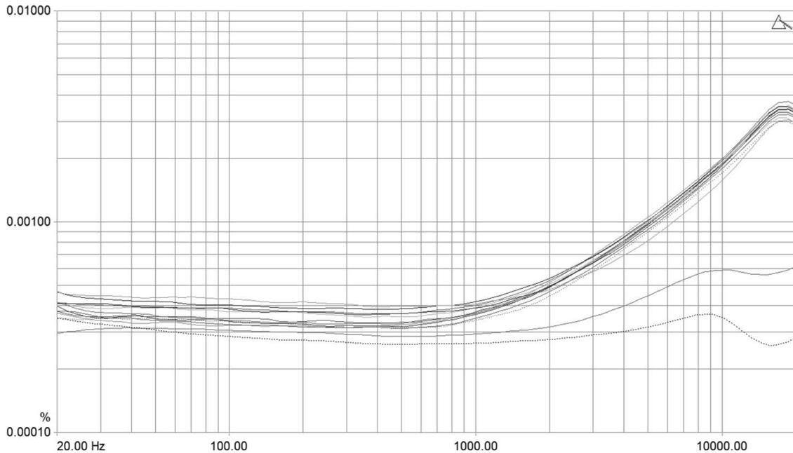
Fig. 6. Total harmonic distortion (THD) sweeps at +20 dBu.
