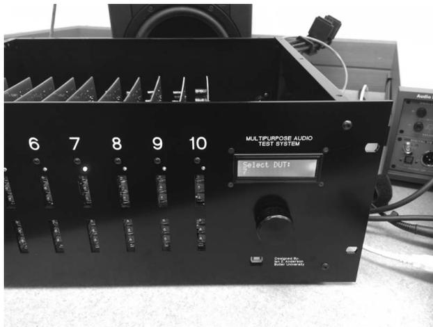
Fig. 2. User interface (UI) and precision trimmer potentiometers.
