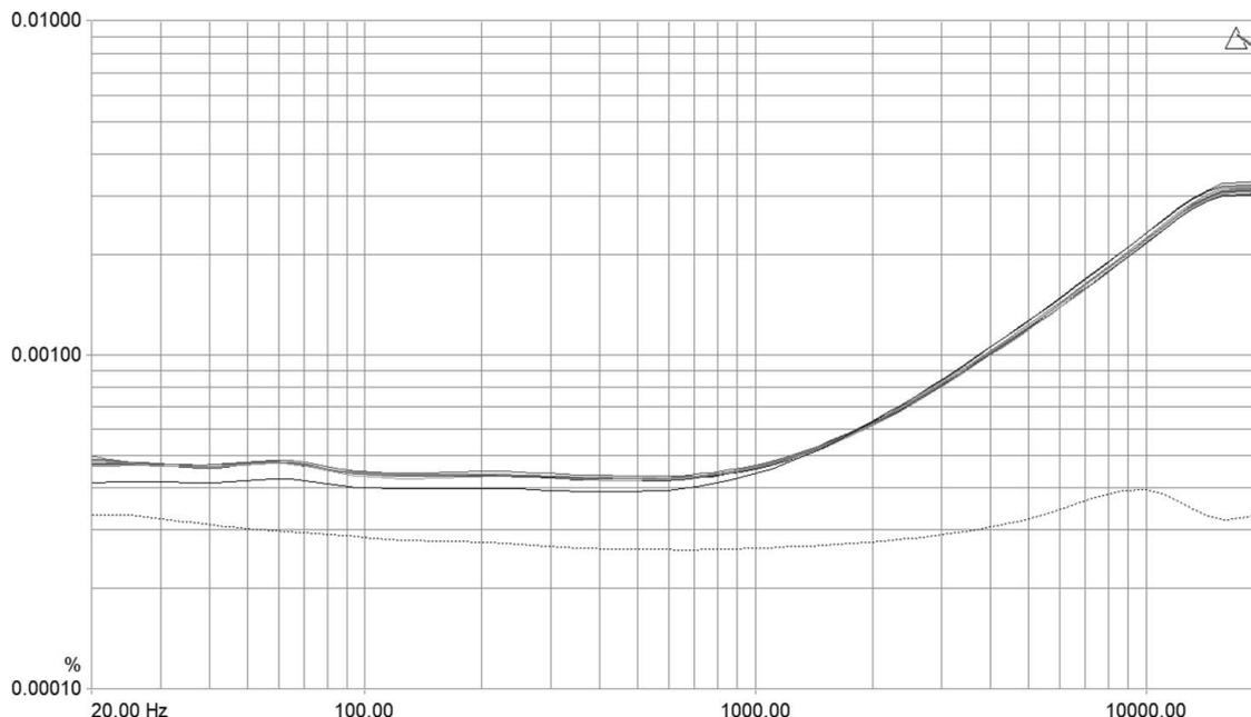
Fig. 7. Total harmonic distortion (THD) sweeps, single-stage unity gain inverting amplifier, +20 dBu.
