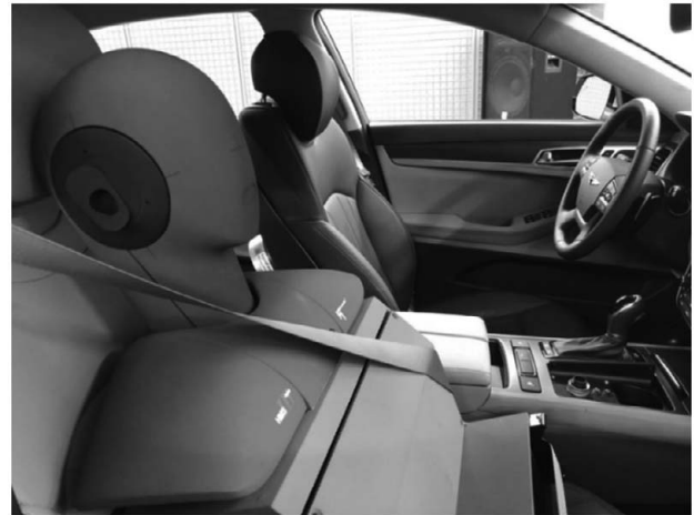
Fig. 2. Example of dummy head setup for engine sound recording.
