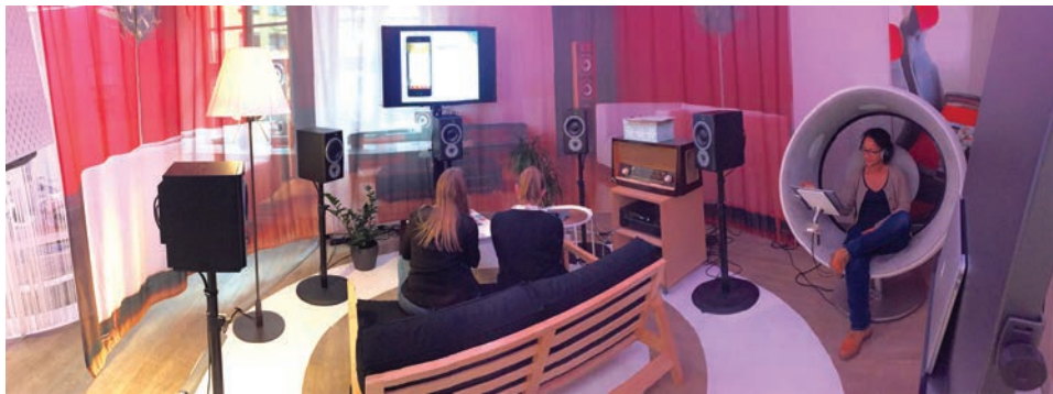
Fig. 5. ORPHEUS test installation at open innovation lab JOSEPHS; left side: loudspeaker reproduction at home; right side: headphone reproduction in a noisy environment (produced by loudspeakers in sonic chair), mobile listening .
