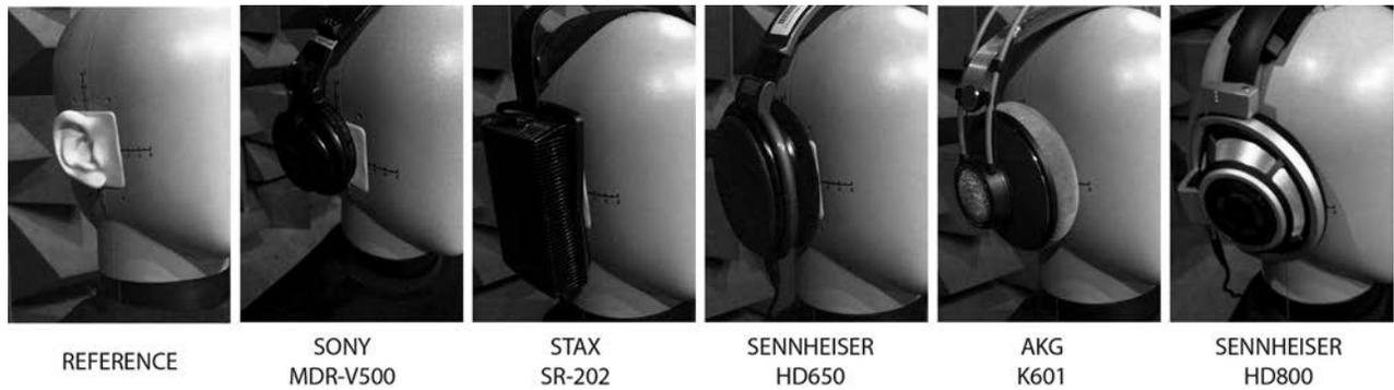
Fig. 1. Headphone sets mounted on B&K HATS for physical measurement stage of the investigation.
