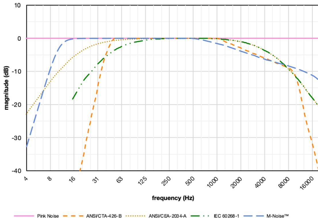
**Figure 0 – RMS spectra of various Simulated Programme Content normalized at 500 Hz**
