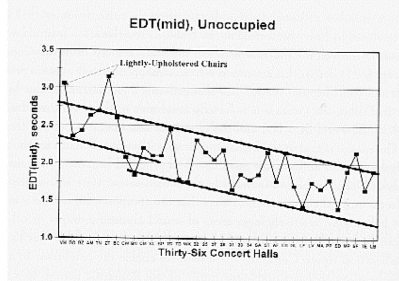
**The right hand graph gives the early decay time EDT plotted against the rank ordering of the halls according to acoustical quality. For judging acoustical quality, it appears that the early decay time, EDT (measured with hall unoccupied) is a better measure than reverberation time. Part of the variation in location of points on the EDT graph is due to different degrees of chair sound absorption.**
