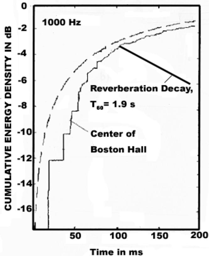
Assume that a violin plays a note 100 ms long with energy in the 1000 Hz band. At a seat in the center of the Boston Hall the cumulative energy will rise as shown by the irregular curve. At 100 ms, the energy will start to decay.
