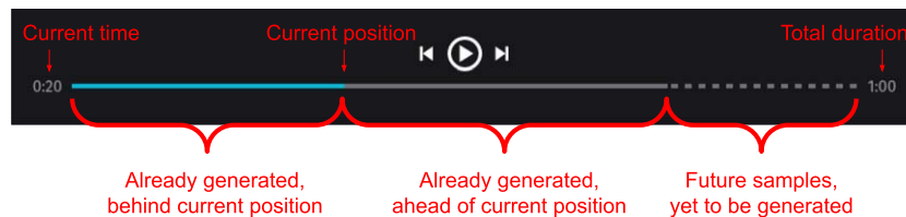
Fig. 4. Alternator extends the visual language of conventional music players for computational music. Seeking to the dashed region, which represents the unknown future, will trigger faster-than-real-time rendering.
