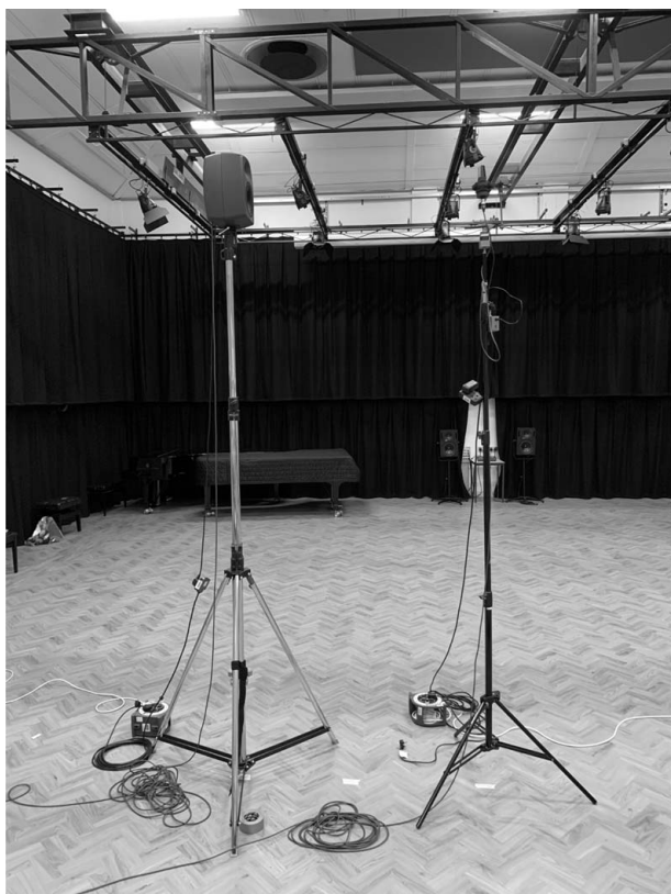
Fig. 2. AKG C414 microphone positioned on-axis at a source-to-microphone distance of 1.25 m.
