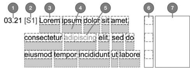
Fig. 2. Layout of the PaperClip interface, which features timestamps at beginning of each paragraph (1), speaker labelling (2), word removal (3), word selection (4), confidence shading (5), line selection (6), and a margin for freehand notes (7). Dotted lines indicate hidden active zones for selection and removal.
