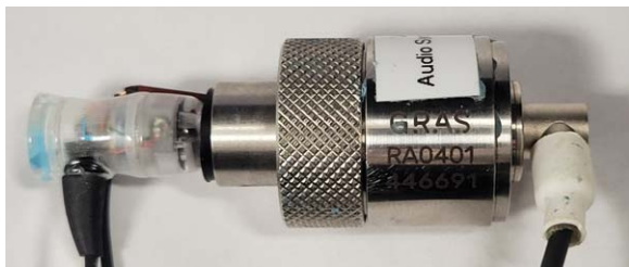
Fig. 5. Headphone measurement using funnel-shaped adapter.
