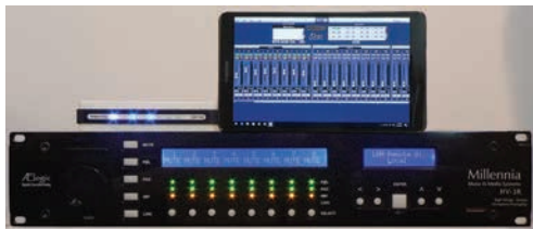
Millennia's HV-3R microphone preamp connected to the Wi-Fi access point with a Galaxy Tab S controlling it
