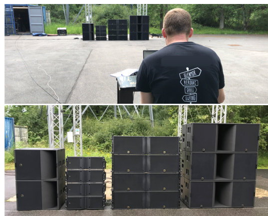
Fig. 4: Overview of the experimental setup and loud-speaker systems, from left to right: KS21 (sub) with KARA II (main), and K2 (main) with KS28 (sub).
