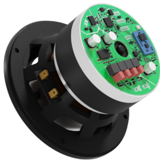
Fig. 8: PCB mounted on the back of the driver
