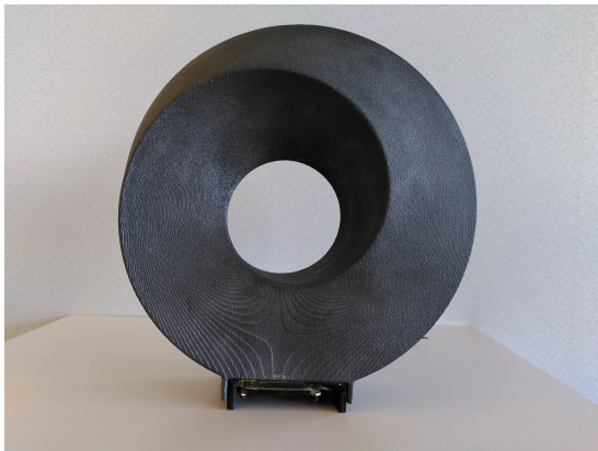
Fig. 1: Initial silicon carbide prototype with driver at bottom position and no reflective element.
