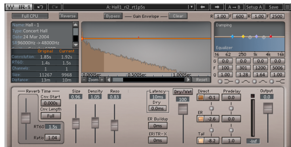
Fig. 4: Plugin 'R1 Convolution Reverb'. The IR selected is the Hall, with a RT 60 = 1.5s.
