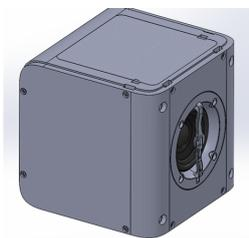
**Fig. 4:** Loudspeaker prototype with NF microphone.
