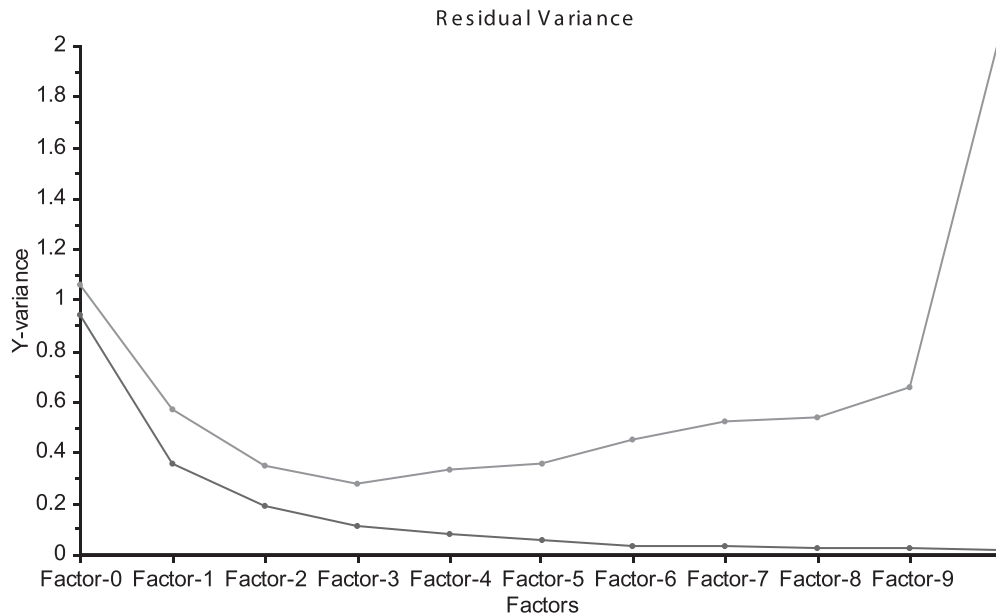
Fig. 8. Residual Y-variance as a function of PLS component number for the iteration that employed 16 metrics and 3 PLS components. The bottom data refer to calibration results, while the top data refer to cross-validation results. Although residual Y-variance was calculated for 16 PLS components, only 10 PLS components are shown for clarity.
