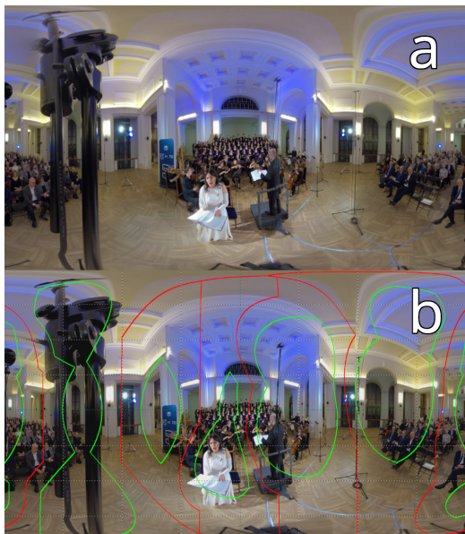
Fig. 7: (a) original, uncorrected stitching with artifacts; (b) the stitching modifications. The red lines indicate the stitching between the recordings from different camera lenses. The green lines indicate the non-stitched areas within which the image originates from a single lens
