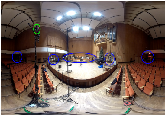
Fig. 2: Ambisonic microphone (green) and spot microphones / individual instrument zones (blue) during the second concert at the Chopin University of Music. The 360 camera is the source of the photo and thus is not visible
