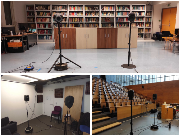
Fig. 2: RIR measurement setups in the three rooms: (top) medium meeting room with omnidirectional source setup, (bottom-left) small office room with directional source setup, (bottom-right): large lecture theatre.
