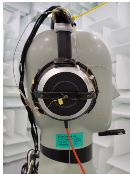
Fig. 2. The hearing device prototype is seen on a HATS. The microphones are connected to external hardware for measurements.
