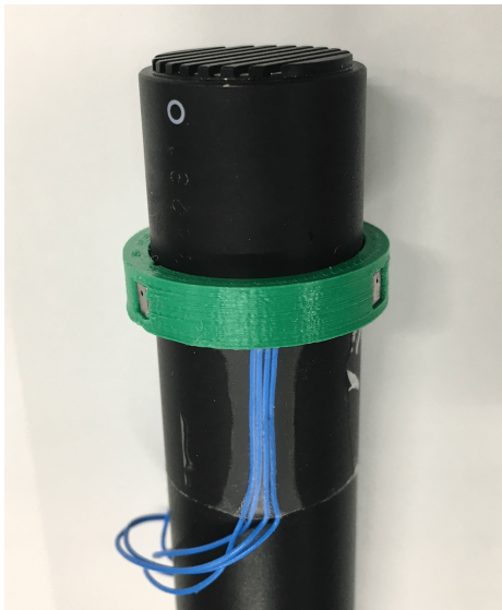
Fig. 3: Prototype of the proposed one-plus-three microphone array configuration, where the high-quality omni-directional capsule is accompanied by three MEMS-microphones (on the 3D printed green ring).
