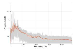
Fig. 8: Noise level calculation using moving median on the spectrum. Light colored lines are the power spectrum of the sound A1, and darker curve is moving median of the spectrum.
