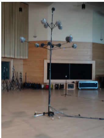
Figure 6 – 8+4+1 Array in Witch's Hat configuration
