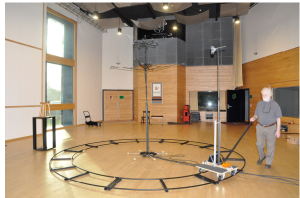
Figure 8 – 360° Rail, Blue Tooth Loudspeaker Sound Source, and 13 channel Top Hat Array under test.
