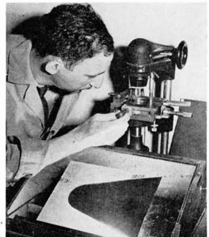
Fig. 3. Each diamond stylus must be inspected carefully on a shadowgraph.
