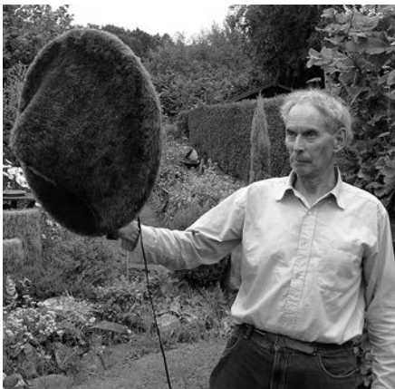
Mike Skeet with an unusual mic system that is actually a parabolic reflector with a DIY Jecklin Disc array at the focus (i.e., a binaural set up), and an Olympus handheld recorder built into the handle. (Photo courtesy Ashley Styles of SATURN SOUND Recording Services.)
