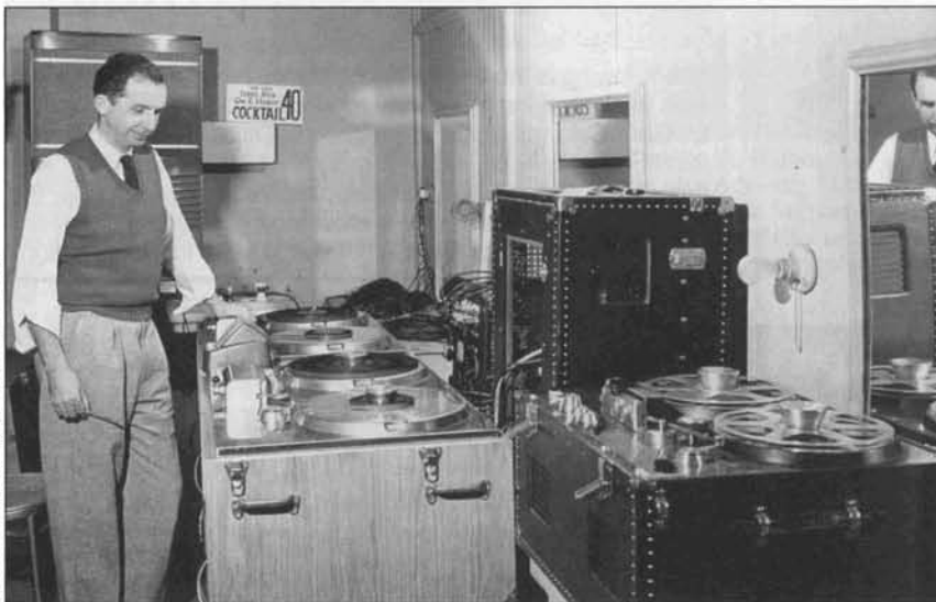
Mullin in an ABC radio network control room with the only two "portable" Ampex Model 200 tape machines ever built (in oak cases on the left). On the right, early portable Model 300 (black case). The Model 200s replaced Mullin's two, well-worn modified AES Magnetophones that put Bing Crosby on tape in 1947.
