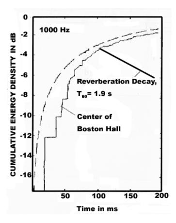
Assume that a violin plays a note 100 ms long with energy in the 1000 Hz band. At a seat in the center of the Boston Hall the cumulative energy will rise as shown by the irregular curve. At 100 ms, the energy will start to decay.
