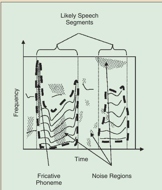
Fig. 3. Noisy speech with segments identified (Figs. 3 and 4 courtesy Maher)
