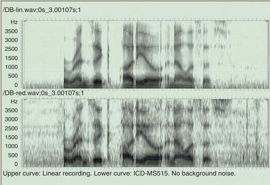
Fig. 2. Comparison of spectrographs of a linear PCM recording and a bit-rate-reduced version of the phrase “forensic audio analysis” (courtesy Brixen and Begault).
