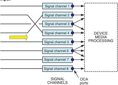
Figure C.5 - Channel-based input
