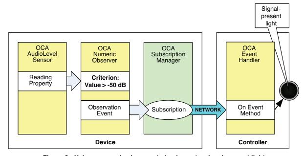
Figure 9 - Using a numeric observer to implement a signal-present light
