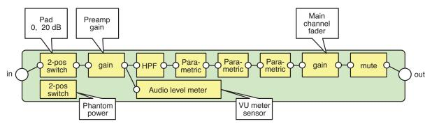
Figure B.3 - Mic channel with EQ sections inline
