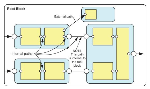
Figure 2 - Signal flow
