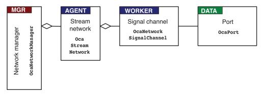
Figure 11 - Channel-based classes
