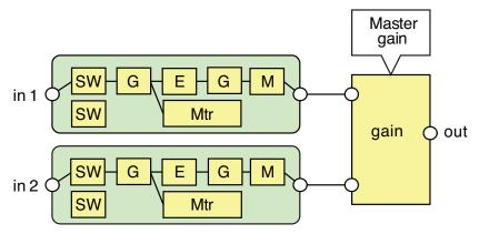
Figure B.2 - Two-channel microphone mixer
