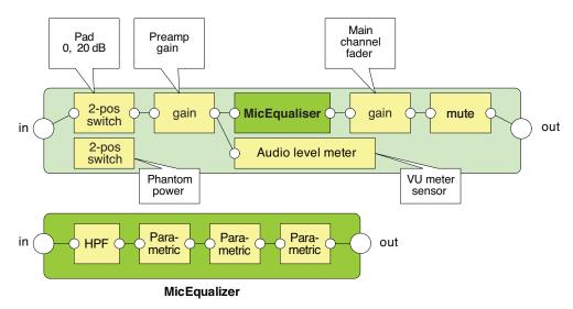
Figure B.4 - Microphone channel with MicEqualizer block
