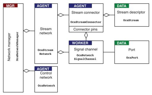
NOTE in this figure, a diamond-headed arrow represents a collection relationship, with the objects at the plain ends being collected by the object at the diamond-headed end.
