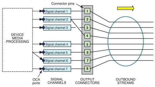
Figure C.2 - Simple stream-based output example
