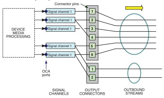
Figure C.3 - Multiple stream-based output connector example
