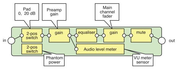
NOTE The illustrations in this document use small circles for Worker ports, large circles for block ports, and simple lines for signal paths. Blocks are shown with rounded corners, other objects with square corners.
