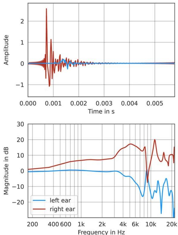
Fig. 7. Example of an HRIR (top) and HRTF magnitude-spectrum (bottom) for a source on the horizontal plane with an azimuth angle of  $270^\circ$  (at the right ear side. The azimuth angle denotes the counter clock-wise angle in the  $x/y$ -plane). HRTFs were calculated for sources at a distance of 1.5 m from the origin of coordinates.
