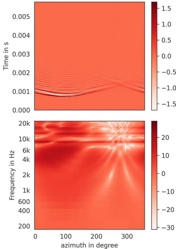
Fig. 8. Example of HRIRs (top) and HRTFs (bottom) of the left ear for sound sources located on the horizontal plane. The azimuth angle denotes the counterclockwise angle in the  $x/y$ -plane. HRTFs were calculated for sources at a distance of 1.5 m from the origin of coordinates.
