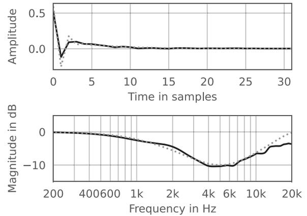
Fig. 9. Example of an inverse DFTF (black, solid) and its approximation by a bell filter (gray, dotted). The bell filter was generated with `pyfar.dsp.filter.bell` using a center frequency of 5 kHz, a gain  $-10$  dB, and a quality 0.75.
