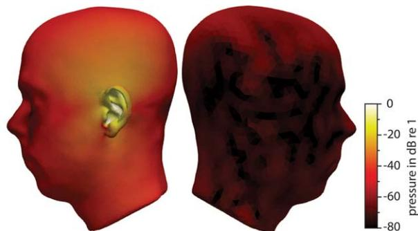
Fig. 5. Example of a left-ear mesh showing the color-coded sound pressure in decibels at 7 kHz. The sound pressure was calculated with NumCalc. The visualization was done with `export.vtk` and ParaView (<https://www.paraview.org/>). The pressure was normalized to 0 dB.
