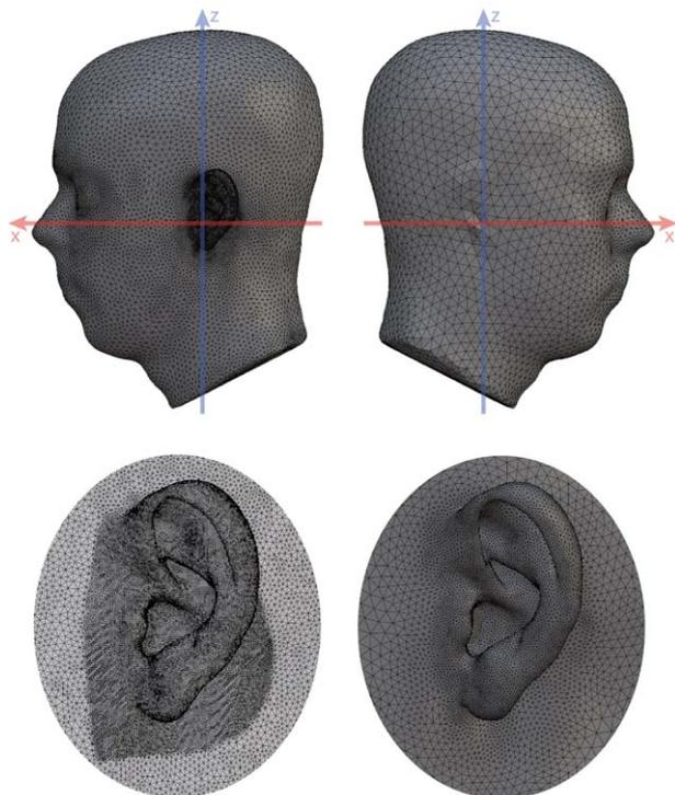
Fig. 2. Illustration of mesh grading. Top: Example of a graded mesh showing a high-resolution left ear (left panel) and a low-resolution right ear (right panel), used to calculate HRTFs of the left ear. Note that the mesh for calculations of the right-ear HRTFs (not shown here) has a high-resolution right ear and a low-resolution left ear. Bottom: Left ear before (left) and after (right) mesh grading. The original mesh is from the HUTUBS HRTF database [42, 43, subject 22].
