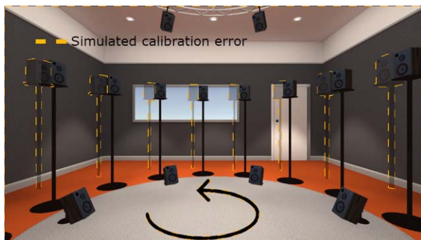
Fig. 6. Visualization of the effect of rotational calibration error, when the integrated SteamVR calibration process is done improperly. Positional and rotational alignment processes of the OMVR platform can help mitigate the effects of calibration errors generated through human error.
