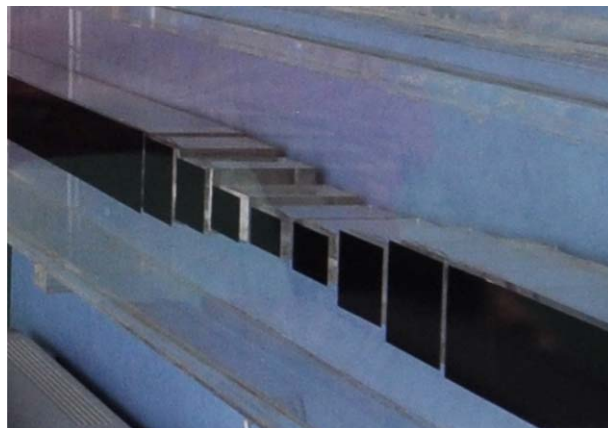
Fig. 6. A Lagasse coupler constructed in transparent acrylic with black tape marking the divide between parallel waveguides and the branch-line section.
