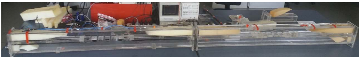
Fig. 3. The AVNA prototype setup with the much larger 1,000–2,000-Hz heads constructed in transparent acrylic. A device under test (DUT) would be inserted between the two couplers at bench level, where the two tables meet. Steel flange screws are just visible in the image.
