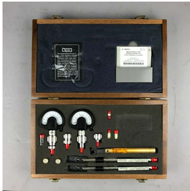
Fig. 11. An Agilent 85056A 2.4 mm VNA calibration kit, including sliding loads and calibration data.
