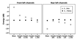
Fig. 8. Results of energy measurements for the direct and ambient sounds of multichannel impulse responses
