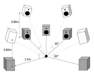
Fig. 2. Loudspeaker setup based on the 9-channel Auro-3D
