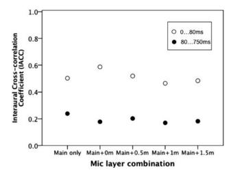
Fig. 11. Interaural cross-correlation coefficients for the binaural impulse responses of height channel reproduction with different vertical microphone spacings; IACC<sub>E3</sub> indicates integration from 0 ms to 80 ms and IACC<sub>L3</sub> from 80 ms to 750 ms.
