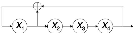
Figure 1 A PRN sequence generating system.
