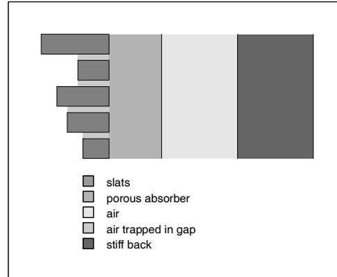
Figure 5 Air transparent diffuser and slat absorber, cross cut
