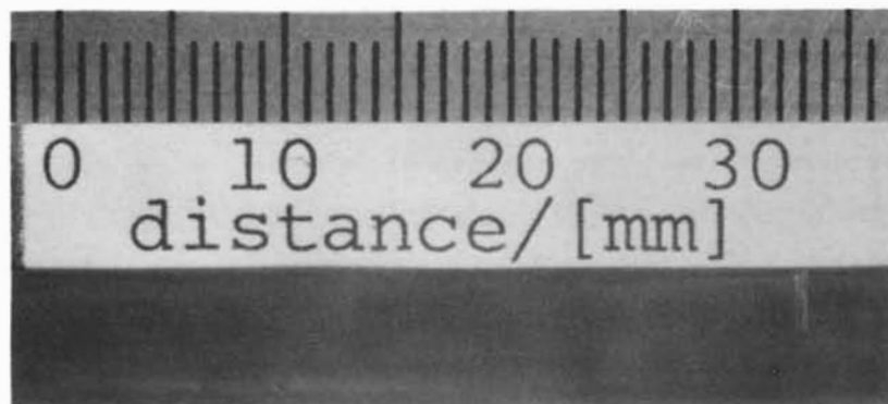
Figure 8. We made this magnetic mark by pushing the RECORDING key of Exhibit 60 Uher and then pushing the STOP key. No tape motion was involved at any time.
