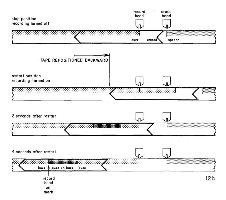
In Figure 12b, the tape is repositioned backward so that the erase and record head marks precede the erase head. Consequently, when recording is resumed, both of these marks will pass by the erase head and be erased. The short segment of tape between the record head and erase head contains a previously recorded buzz that the recording head will overwrite with new buzz.
