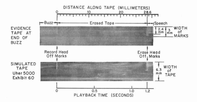
Figure 2. Magnetic marks observed on the Evidence Tape and simulated by using the Exhibit 60 Uher 5000 recorder
