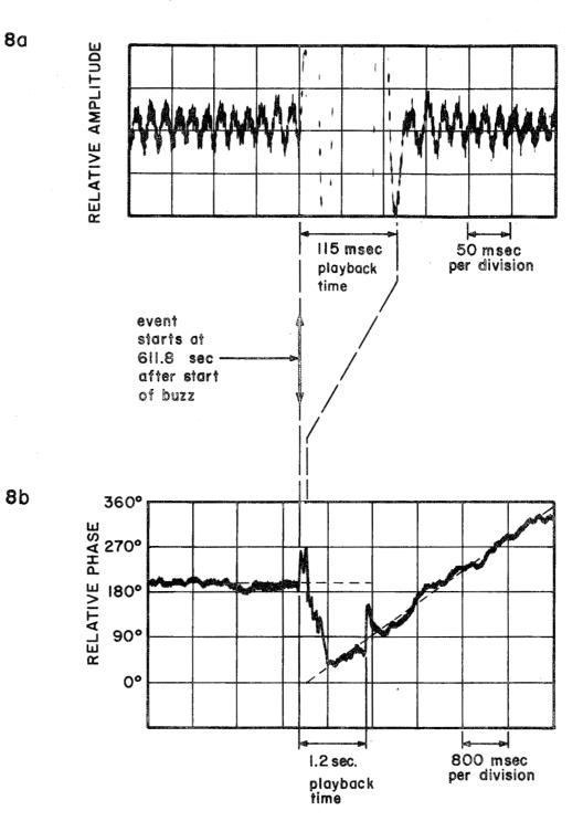
Figure 8. Phase continuity tests on a section of the Evidence Tape starting at 611.8 seconds after the beginning of the buzz.a) Waveform versus time.b) Phase versus time.
