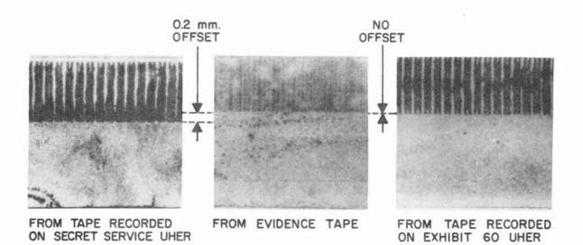
Figure 4. Track offset shown by magnetic marks
