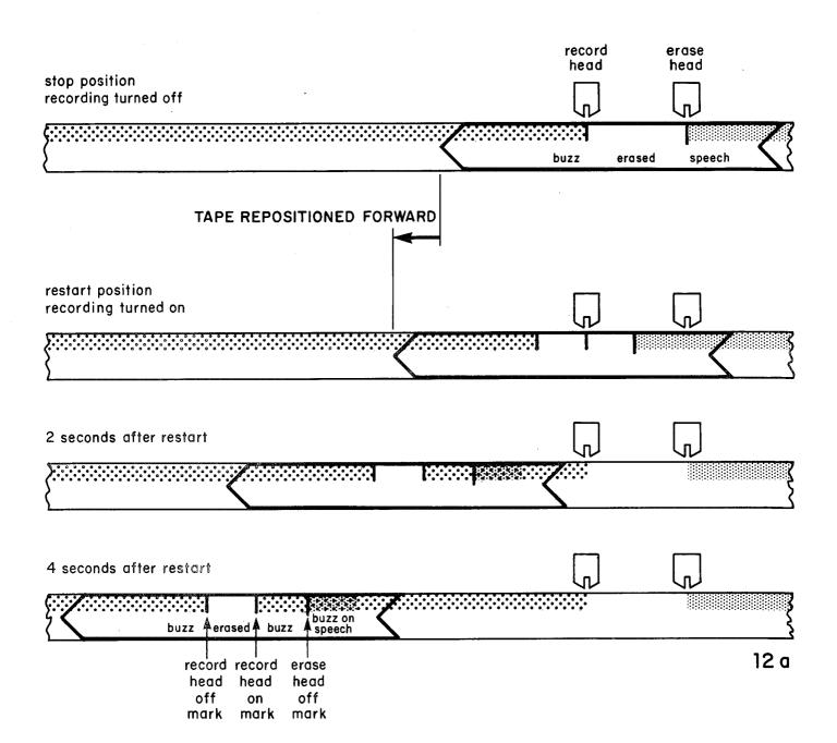
Figure 12. The diagrams represent a section of tape at four positions relative to the record head and erase head of a recorder. As the tape moves in from the right, the erase head obliterates speech recorded previously and the record head puts a buzz sound on the erased tape. In Figures 12a and 12b, the top drawing shows the tape stopped. Record-head-off marks and erase-head-off marks have been written on the tape.
