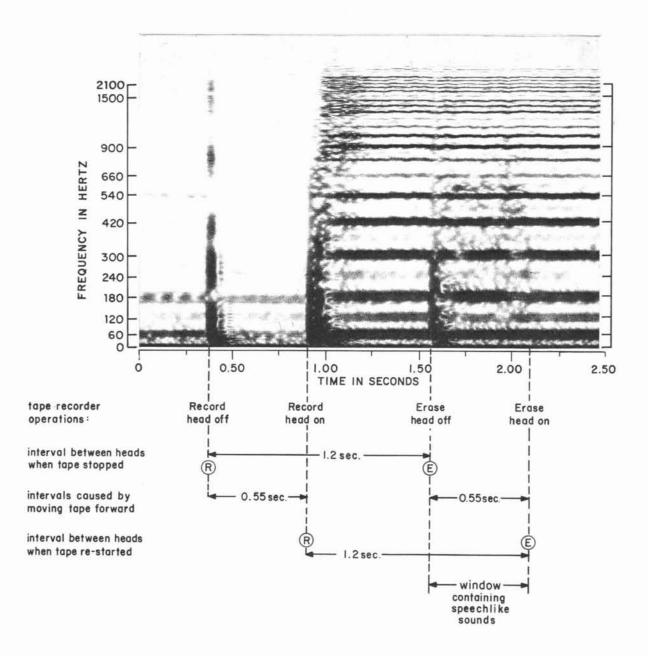
Figure 7. Spectrogram of the buzz starting at about 1041 seconds
