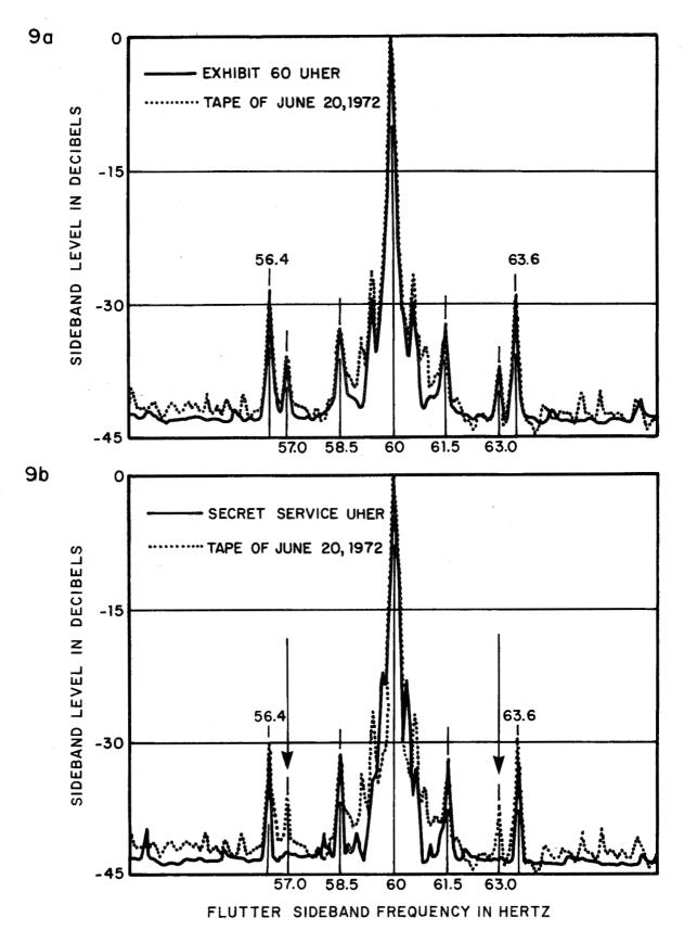
Figure 9. Flutter sideband spectra of the buzz section of the Exhibit Tape. a) Compared with the Exhibit 60 Uher.
