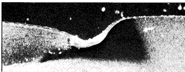
FIGURE 9. MICROSCOPIC VIEW OF A DAMAGED EDGE. AFFECTED AREA EXTENDS ABOUT 15 MILS INTO TAPE.
