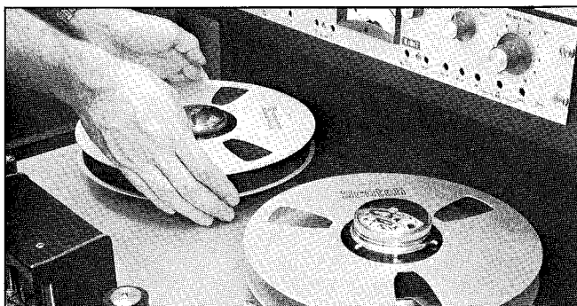
FIGURE 10. PROPER METHOD OF MOUNTING A REEL ON A DECK. APPLY PRESSURE TO THE HUB AND NOT THE FLANGES.
